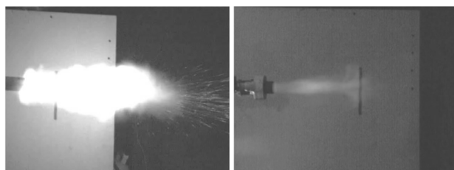
Fig. 12 Photographs of the predetonator nozzle plume at a) detonation failure and b) successful detonation initiation.
